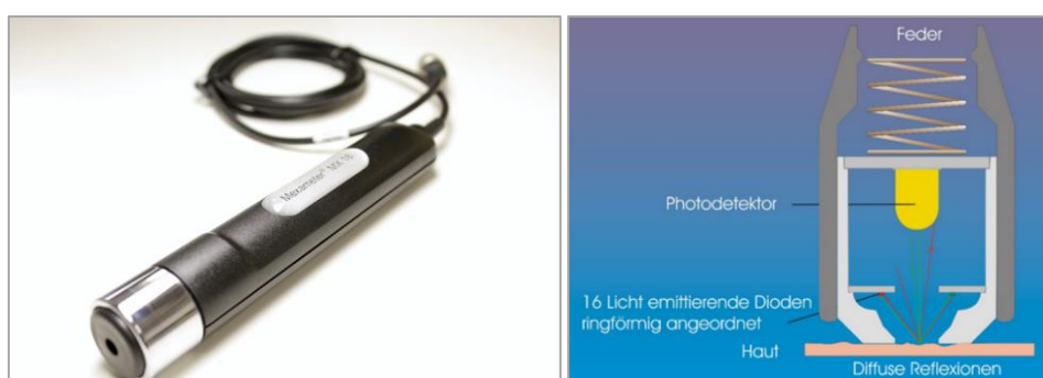
Figure 5. Mexameter® MX18 Device and Measurement Principle
